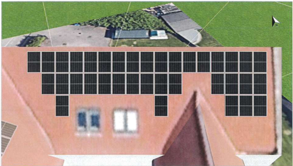
Figure: 2. Module Area - Building 01 - Large South-Roof Area Southwest
